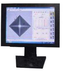
Advanced HV / HK Micro Hardness Indentation Measurement and Analysis system support automatic work mode and manual work mode. And can generate test report in word / Excel format directly, report data including indentation image, hardness value, test force, dwell time, hardness curve, indentation depth, etc.
